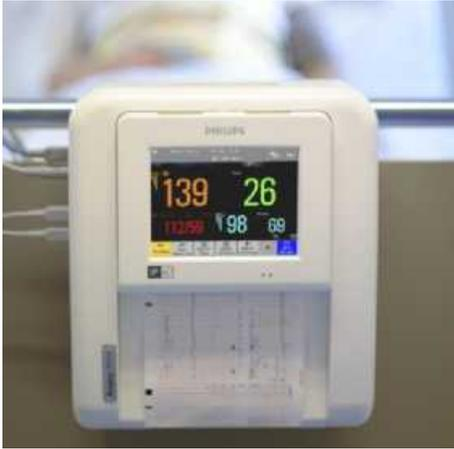
Battery option enables continuous monitoring during maternal transport in healthcare facilities.
